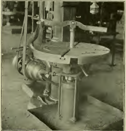
Fig. 3—Pneumatic Clamp for Drill Press.
